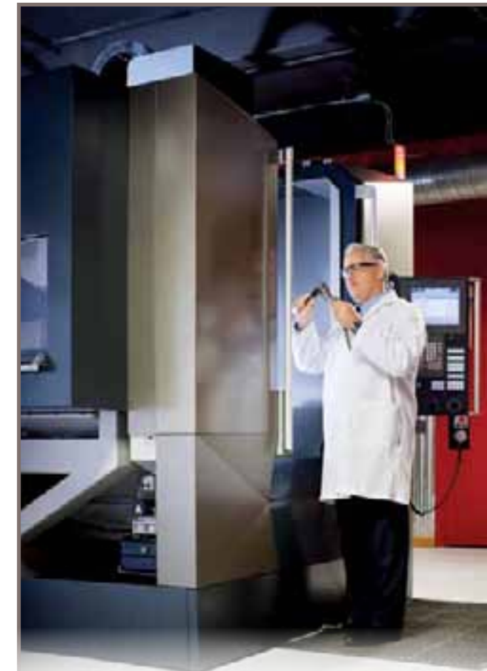
Engineering concepts are converted to prototypes using ABIA's 5-axis vertical milling machine. The machine can create complex shapes out of a multitude of materials ranging from steel to polypropylene.
