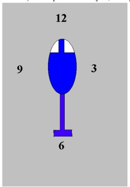
Not all tail rotors are shielded. Stay well clear of an actively spinning tail rotor at the rear (6 o'clock) position of the aircraft
